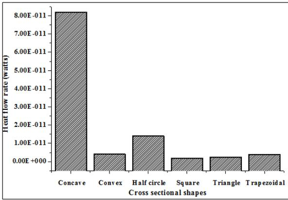
Fig. 15. Heat flow rates of AL200 material for different shapes.
