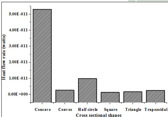
Fig. 17. Heat flow rates of CE17M material for different shapes.
