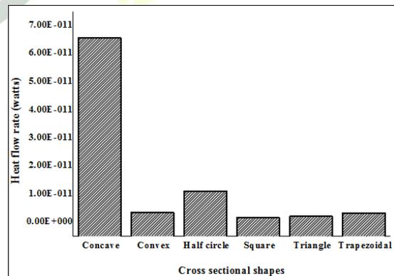
Fig. 14. Heat flow rates of AL6061 material for different shapes.
