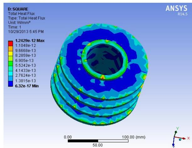
Fig. 8. Conduction analysis surfaces of straight fins.
