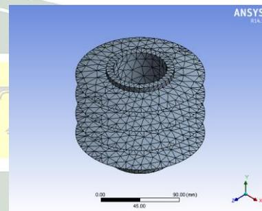
Fig. 4. Volume mesh of half circular shape.
