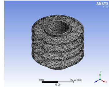
Fig. 3. Volume mesh of concave shape.
