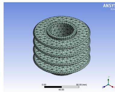
Fig. 6. Volume mesh of triangular shape.
