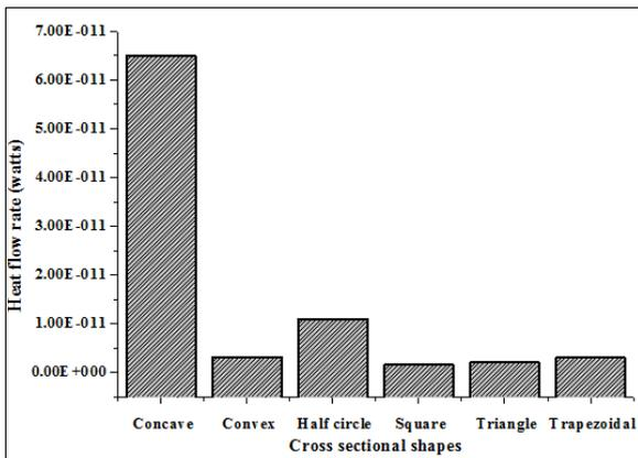
Fig. 16. Heat flow rates of CE17 material for different shapes.
