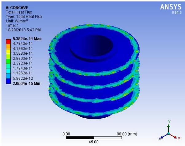
Fig. 9. Conduction analysis surfaces of straight fins.
