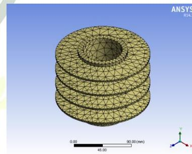
Fig. 5. Volume mesh of trapezoidal shape.
