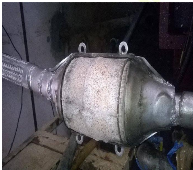
Fig. 4. Photographic view of nanoparticles coated catalytic converter.
