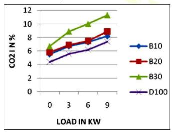
Fig. 8. Variation of carbon-di-oxide (CO2) emission.
