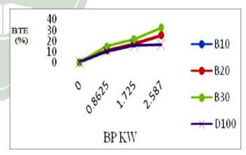
Fig. 5. Effect of brake thermal efficiency for various blends.
