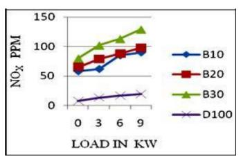
Fig. 6. Variation of nitrogen oxide (NOx) emission.
