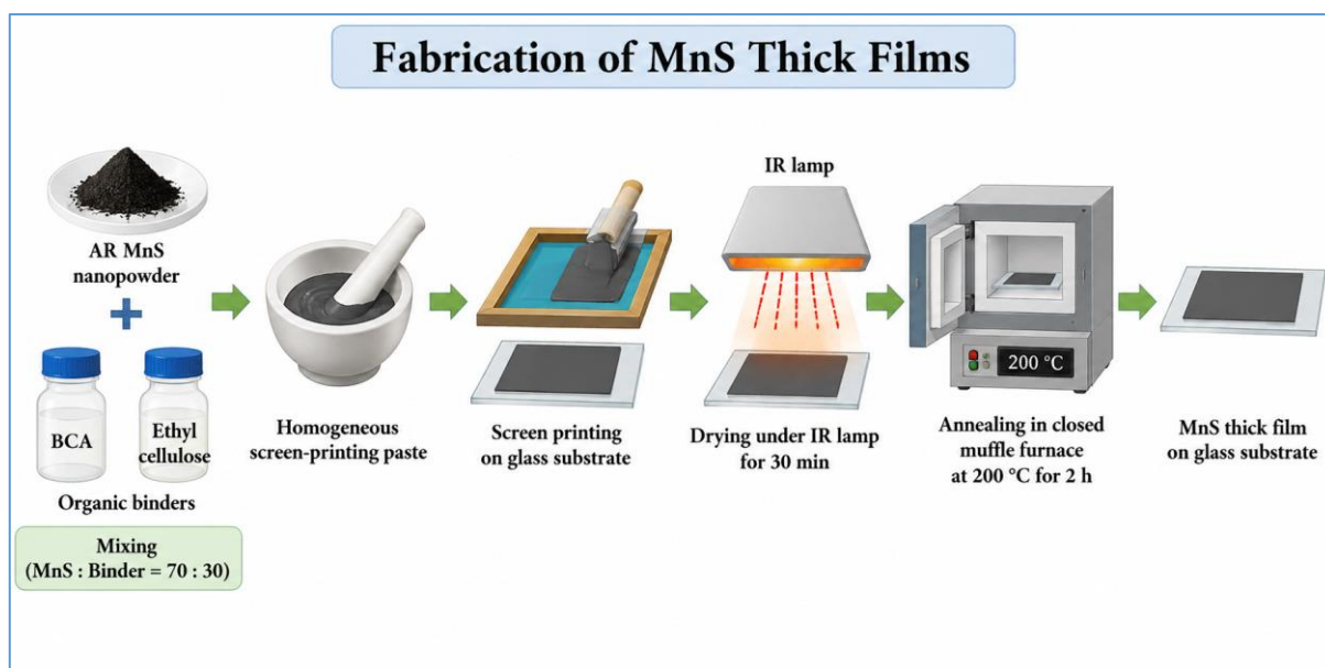
Figure 1: Steps of fabrication of MnS thick films
