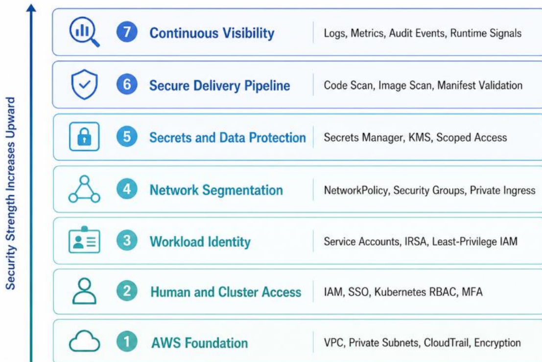
Figure 1. Layered Zero Trust model for production-ready Amazon EKS environments.
