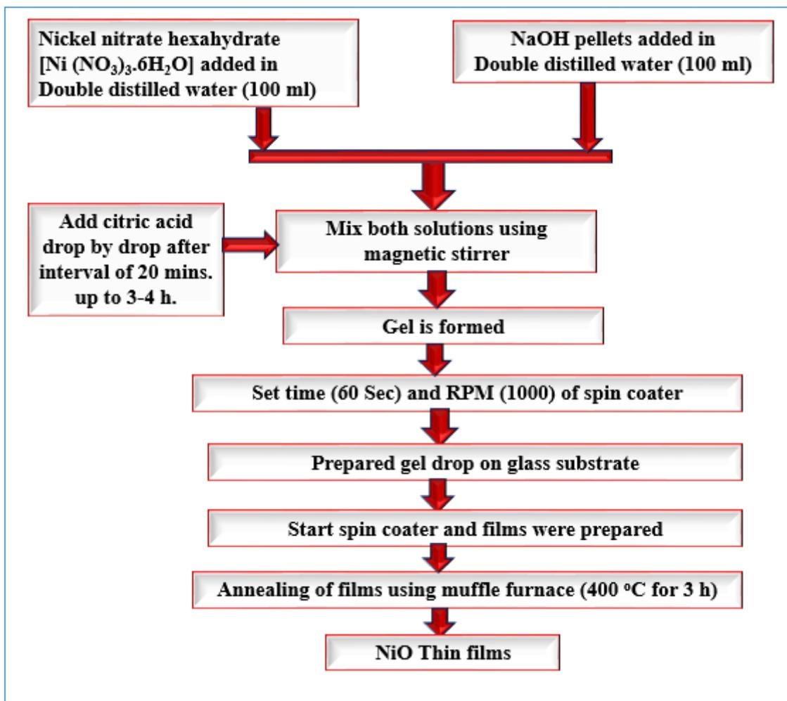
**Figure 1. Steps for synthesis and thin film preparation of NiO**
