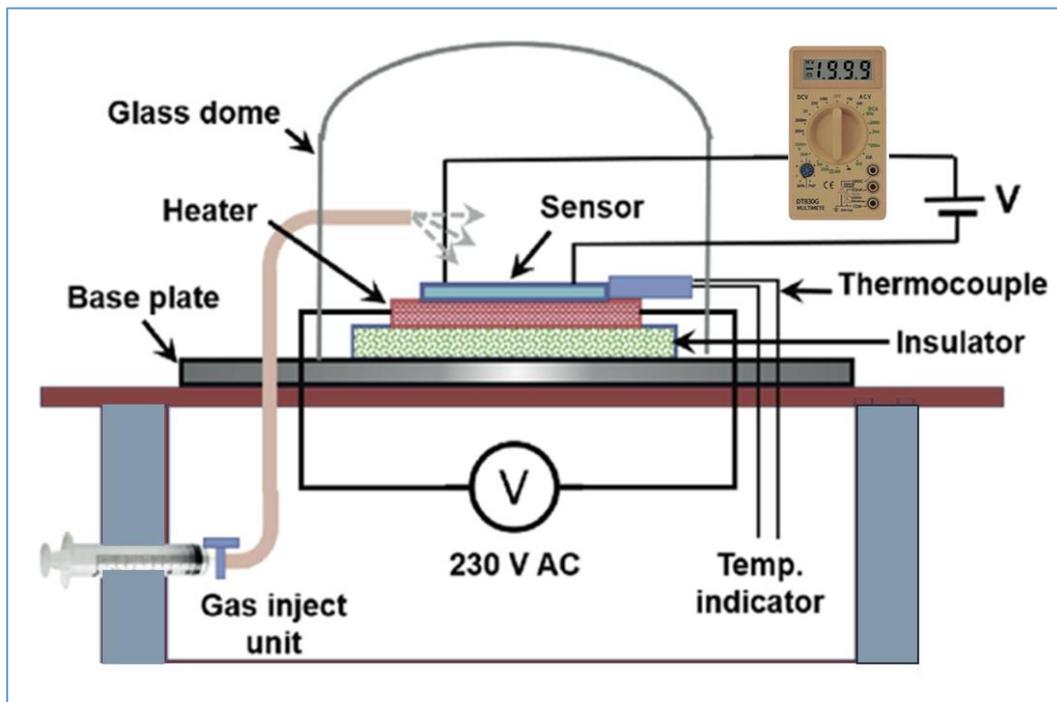
Figure 2. Schematic diagram of gas sensing set-up
