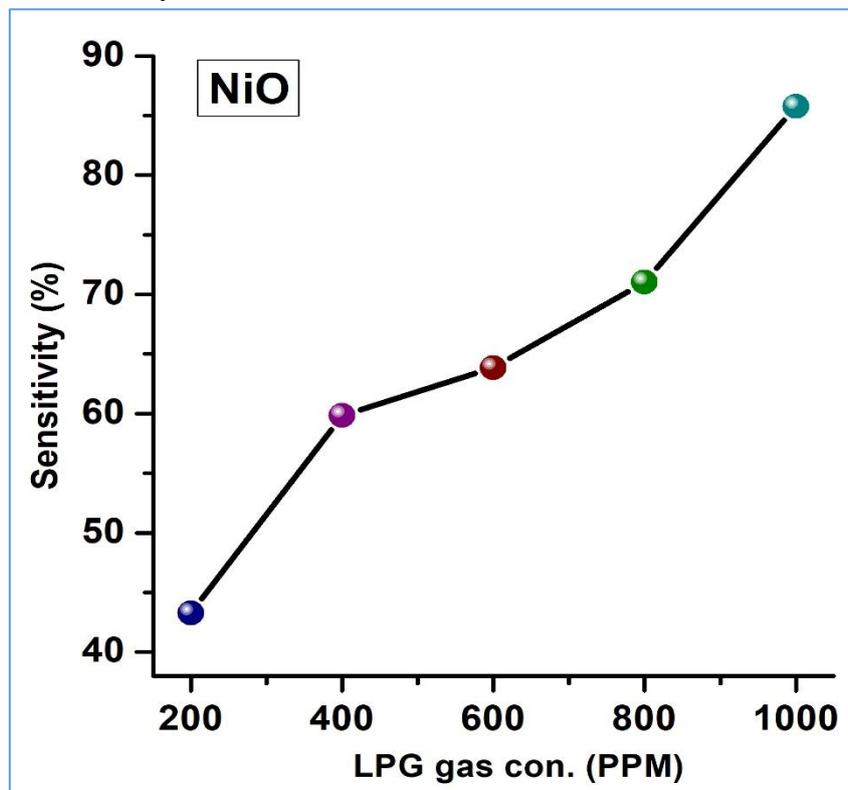
**Figure 4. Sensitivity versus LPG gas concentration plot of NiO thin films**
