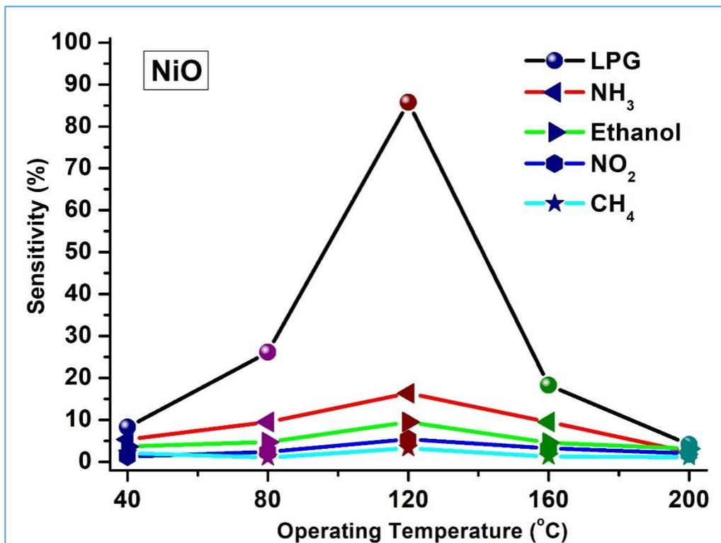
Figure 3. Sensitivity versus operating temperature plot of NiO thin films
