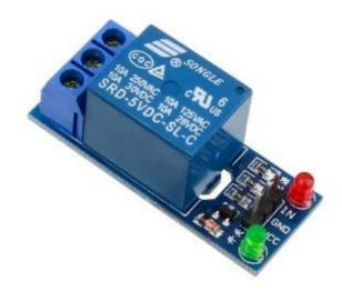
There need to be no electrically operated switch. Current flowing via the relay coil creates a magnetic discipline that attracts the bar and changes the transfer contact. The coil present day can be turned on or off, so the slider position has two positions and is a double function (toggle) transfer. Allow one circuit to bypass
