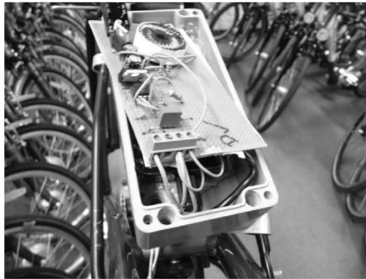
Fig. 6 SEMS electronics, the IOIO board and the Android phone are housed in a water-proof box and are wired into the e-bike battery
