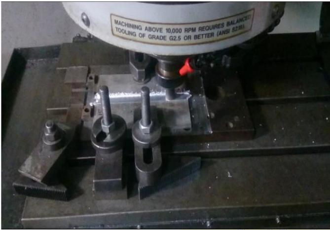
Fig. 3. Work piece set up during FSP.
