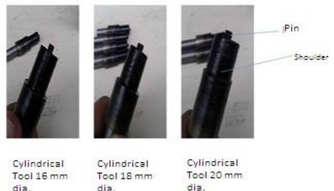
Fig. 2. Processing Tool Pin profiles.
