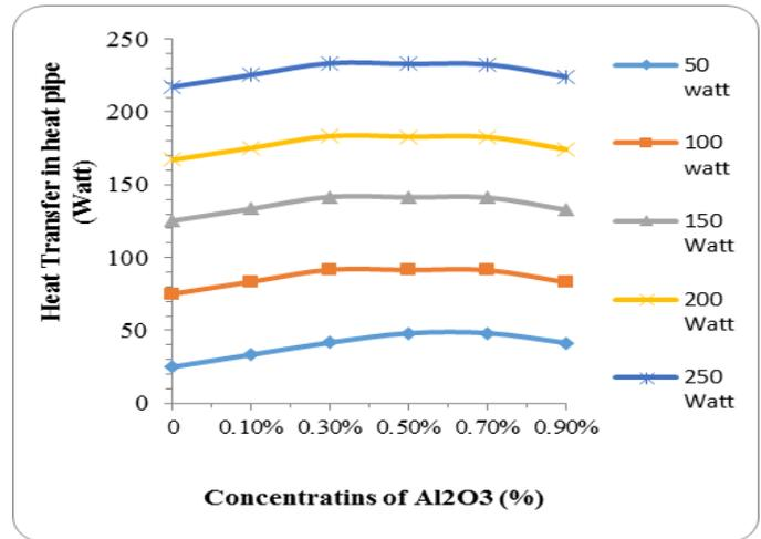
Fig. 1. Variation of heat transfer in heat pipe with  $\text{Al}_2\text{O}_3$  concentrations.
