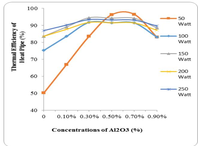
Fig. 4. Variation of thermal efficiency of heat pipe with concentrations of  $\text{Al}_2\text{O}_3$ .
