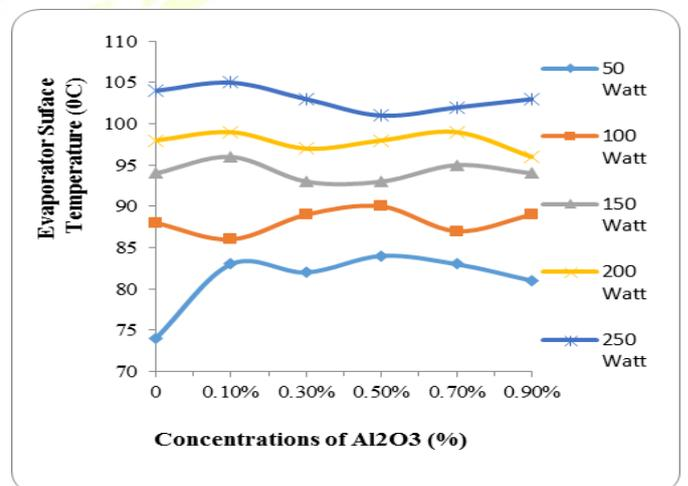
Fig. 2. Variation of evaporator surface temperature with  $\text{Al}_2\text{O}_3$  concentrations.
