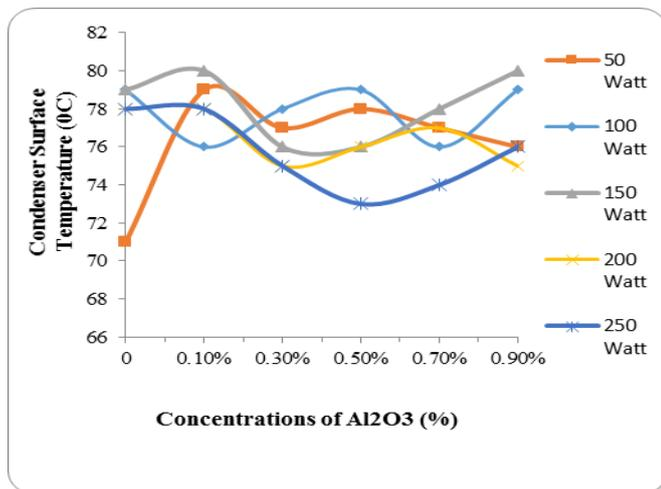
Fig. 3. Variation of condenser surface temperature with  $\text{Al}_2\text{O}_3$  concentration.
