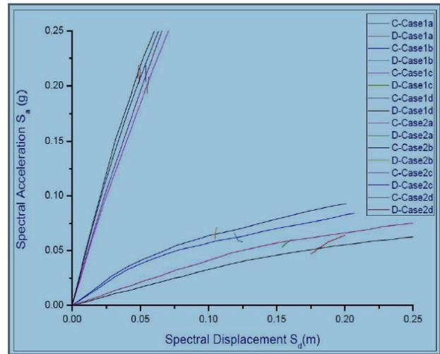
Fig. 11. Comparison of pushover curves of all models considered.
