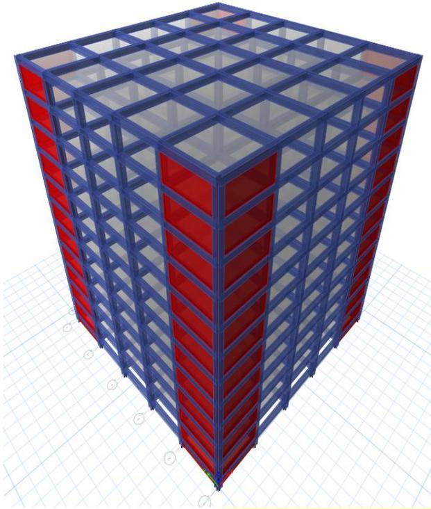
Fig. 2. 3D model of conventional slab-beam-column system with shear wall.
