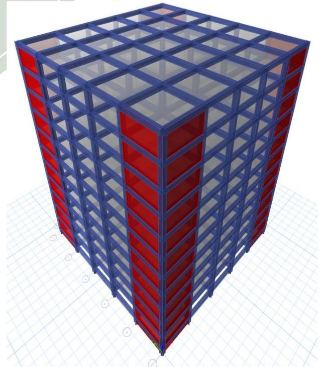
Fig. 1. 3D model of conventional slab-beam-column system without shear wall.
