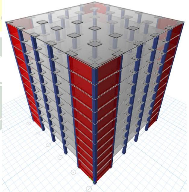
Fig. 9. 3D model of flat slab without edge beam & with shear wall.
