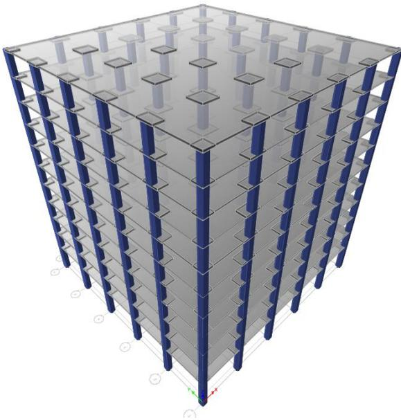
Fig. 7. 3D model of flat slab without edge beam & without shear wall.
