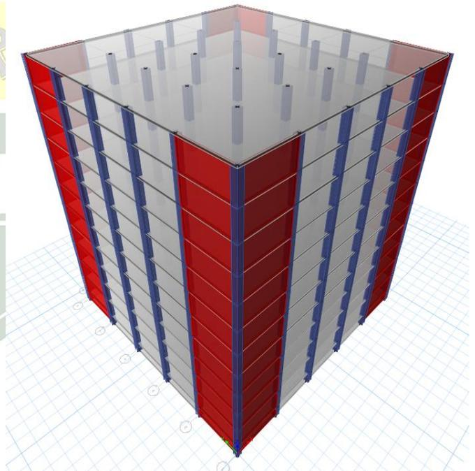
Fig. 5. 3D model of flat plate without edge beam with shear wall.
