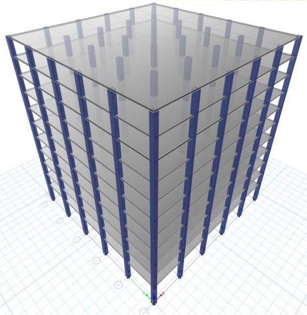
Fig. 3. 3D model of flat plate without edge beam without shear wall.
