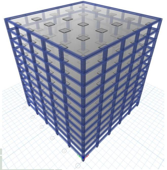
Fig. 8. 3D model of flat slab with edge beam & without shear wall.
