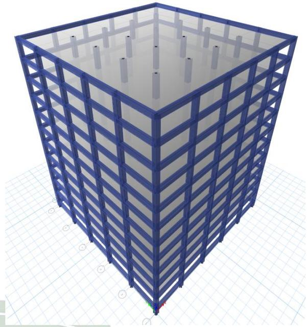
Fig. 4. 3D model of flat plate with edge beam without shear wall.
