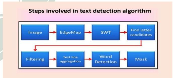
Fig. 5. Text detection algorithm.
