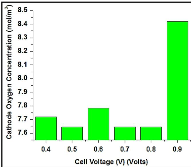
Fig. 3. Cathode Oxygen concentration for all cell potentials.
