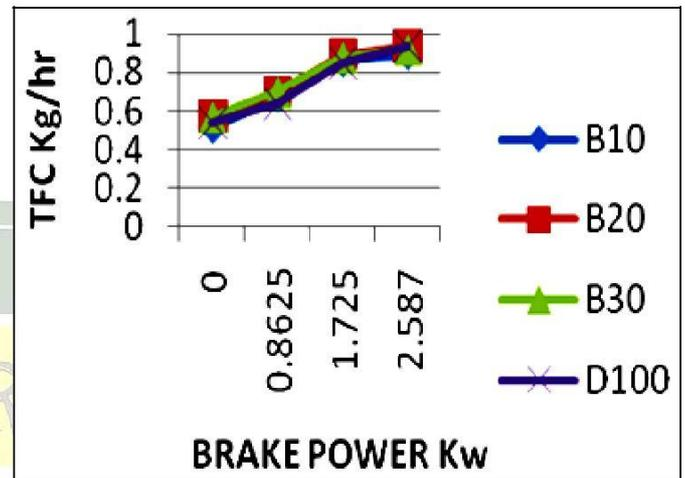
Fig. 4. Effect of Total Fuel Consumption for various blends.
