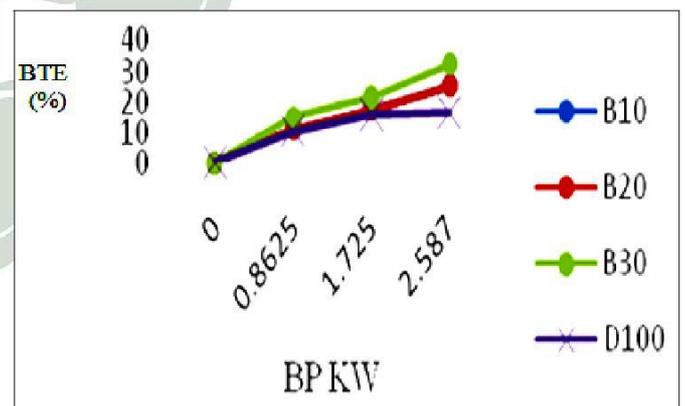
Fig. 5. Effect of brake thermal efficiency for various blends.
