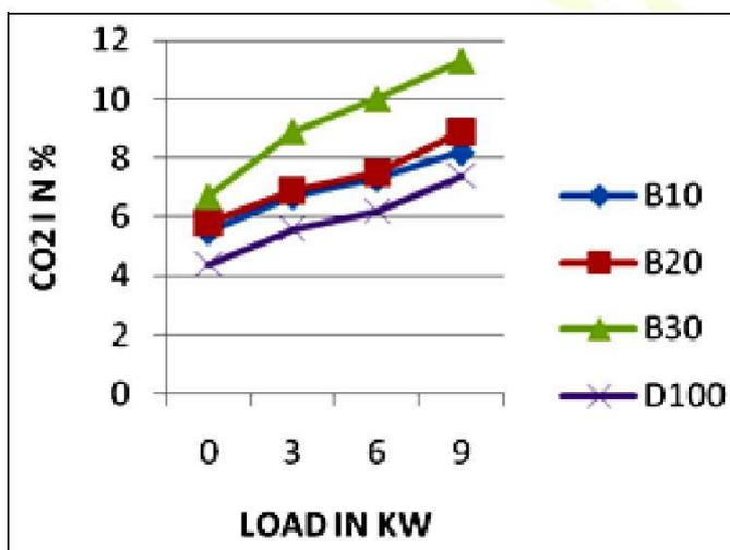
Fig. 8. Variation of carbon-di-oxide (CO2) emission.
