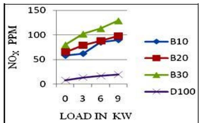
Fig. 6. Variation of nitrogen oxide (NOx) emission.
