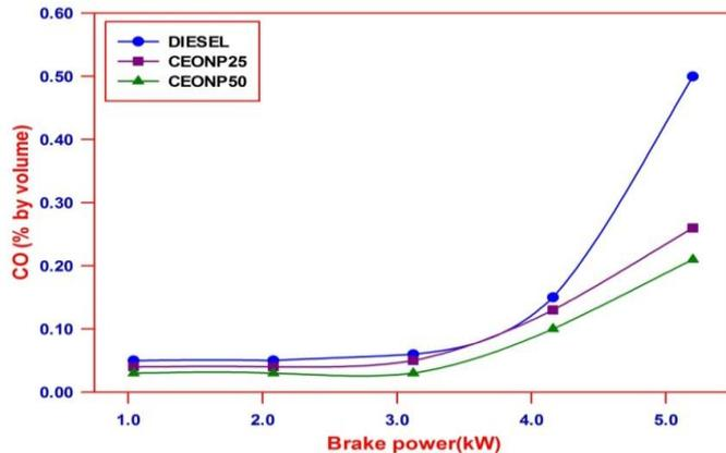
Fig. 9. Carbon monoxide emission against Brake Power.
