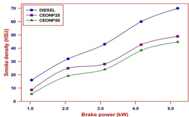
Fig. 8. Smoke density against Brake Power.
