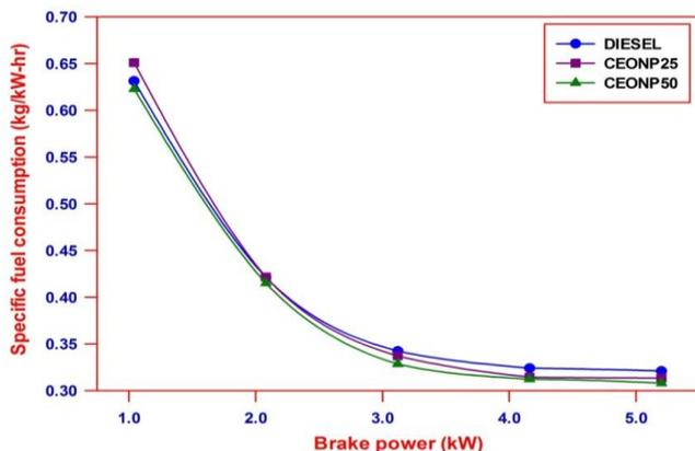
Fig. 6. Specific fuel consumption against Brake Power.
