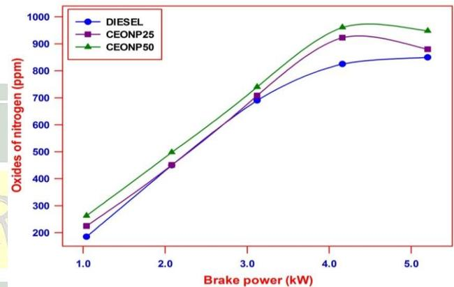
Fig. 7. Oxides of nitrogen against Brake Power.
