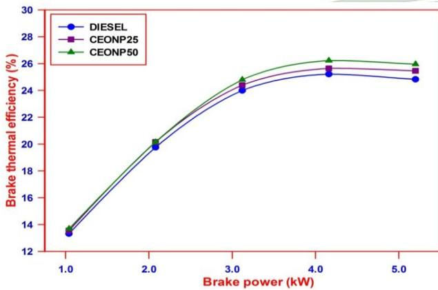
Fig. 5. Brake thermal efficiency against Brake Power.
