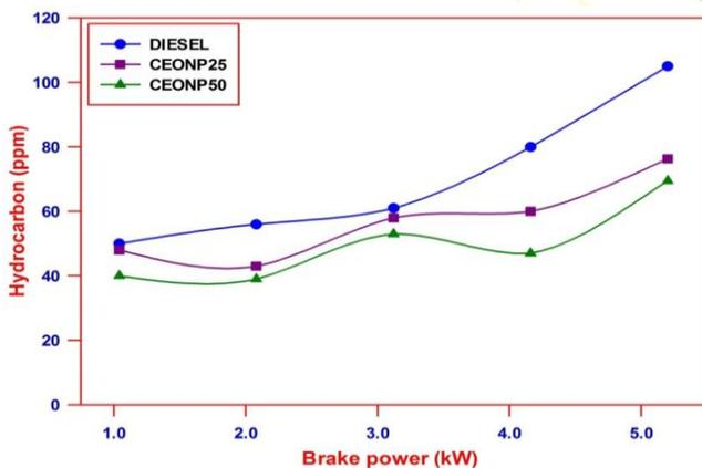
Fig. 10. Hydrocarbon emission against Brake Power.
