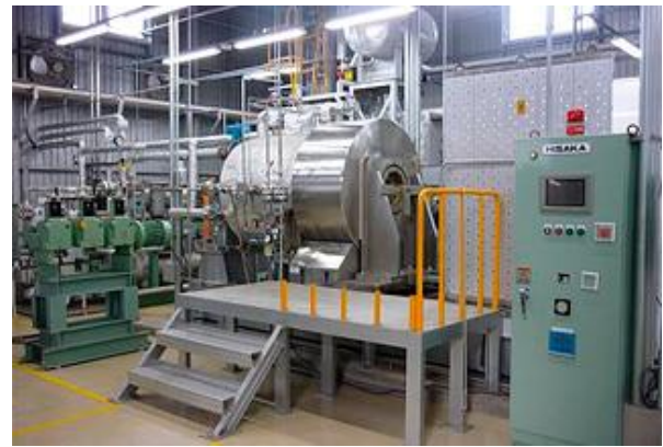
Fig. 3. A typical dyeing apparatus for CO 2 assisted dyeing
