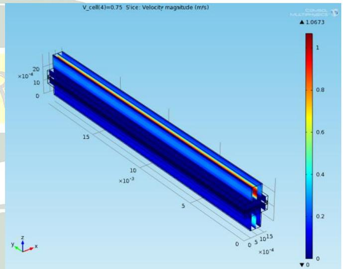
Fig.9. Reactant gases flow velocity at 0.75V
