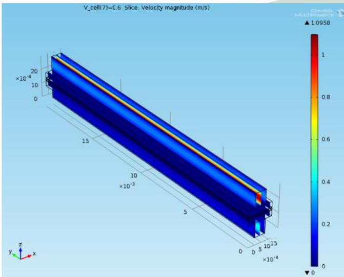
Fig.6. Reactant gases flow velocity at 0.6V
