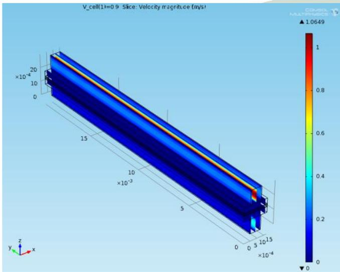
Fig.12. Reactant gases flow velocity at 0.9V
