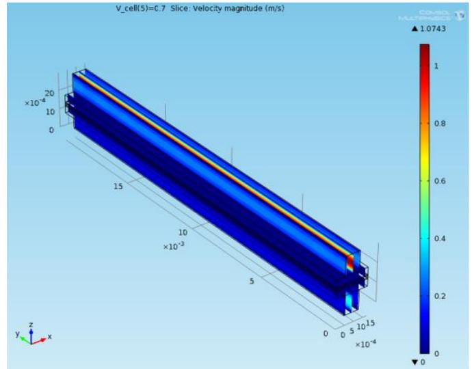
Fig.8. Reactant gases flow velocity at 0.7V
