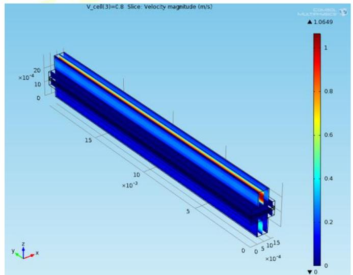
Fig.10. Reactant gases flow velocity at 0.8V
