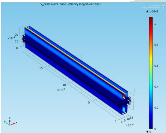
Fig.12. Reactant gases flow velocity at 0.9V
