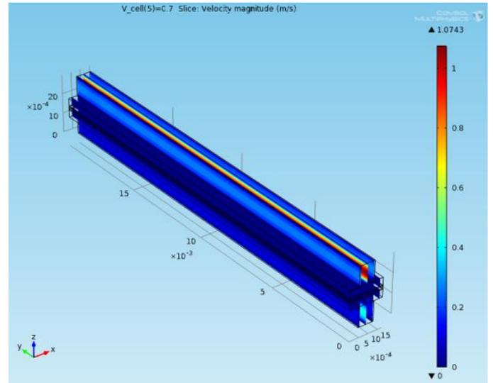
Fig.5. Reactant gases flow velocity at 0.55V
