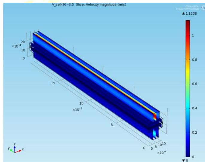
Fig.4. Reactant gases flow velocity at 0.5V
