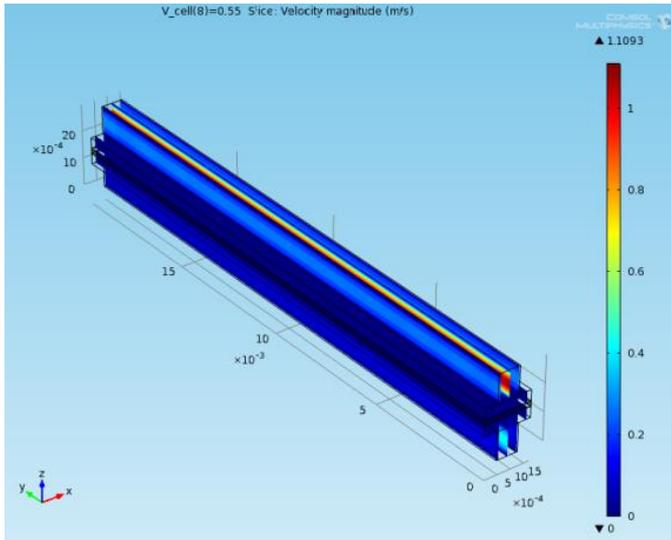
Fig.5. Reactant gases flow velocity at 0.55V
