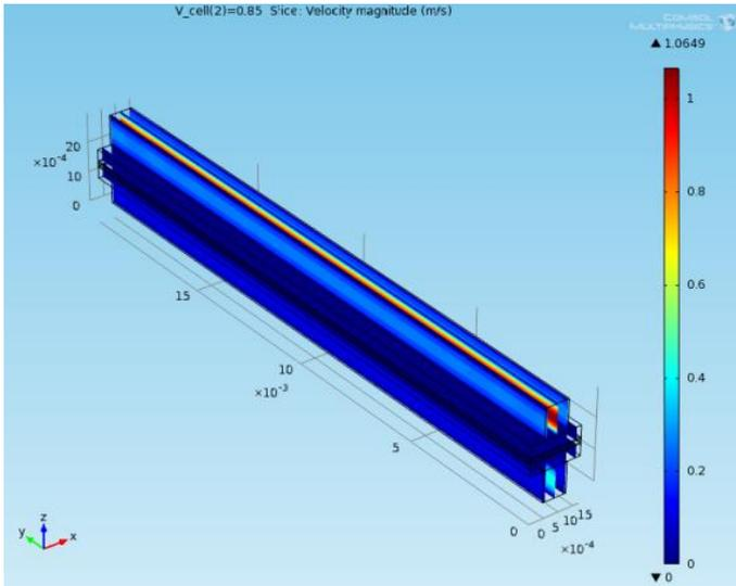
Fig.11. Reactant gases flow velocity at 0.85V
