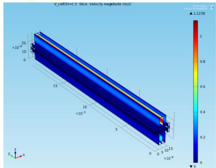
Fig.4. Reactant gases flow velocity at 0.5V
