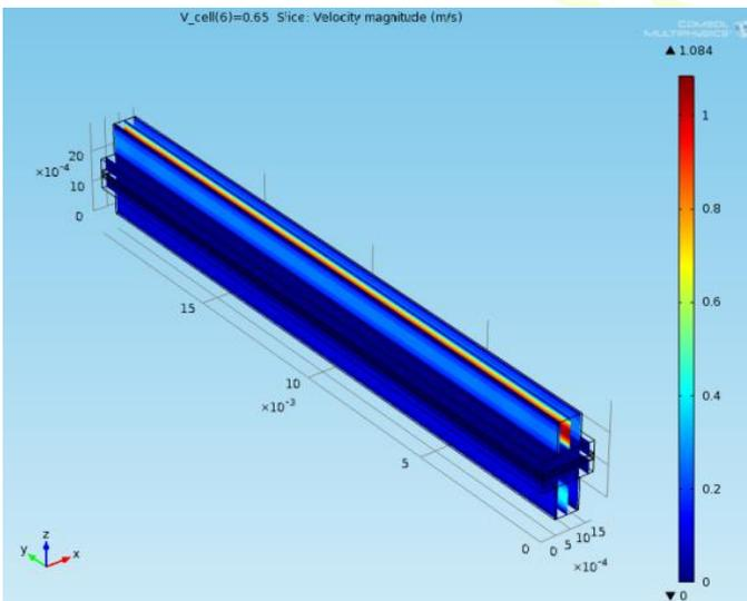
Fig.7. Reactant gases flow velocity at 0.65V
