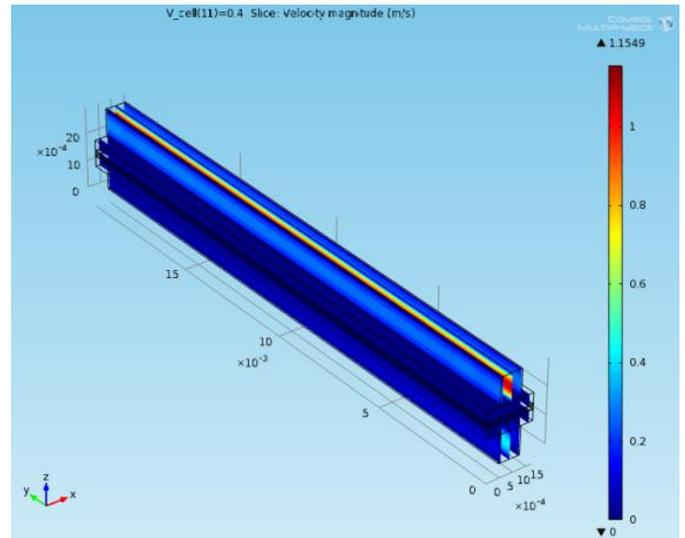
Fig.2. Reactant gases flow velocity at 0.4V
