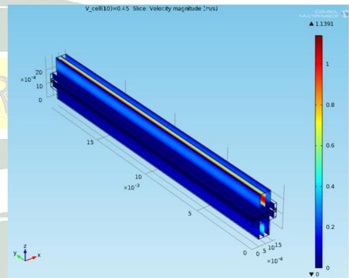
Fig.3. Reactant gases flow velocity at 0.45V
