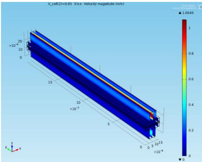
Fig.11. Reactant gases flow velocity at 0.85V
