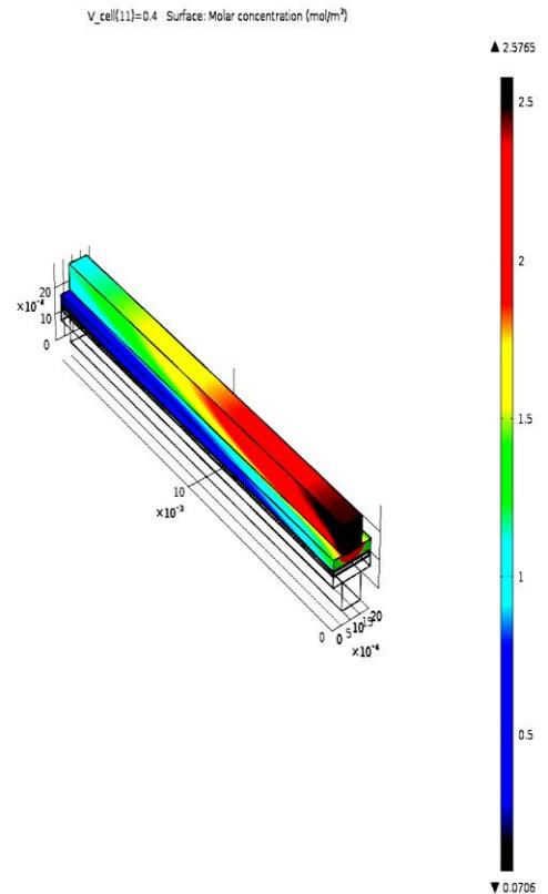
Fig.4. Cathode oxygen concentration at 473K
