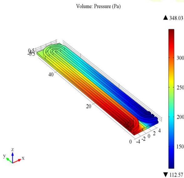
Fig.11. Gas diffusion layer pressure distribution at 0.45 V
