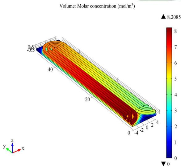
Fig.22. Cathode oxygen concentration at 0.35 V
