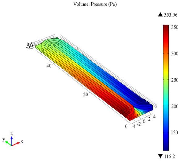
Fig.9. Gas diffusion layer pressure distribution at 0.25 V
