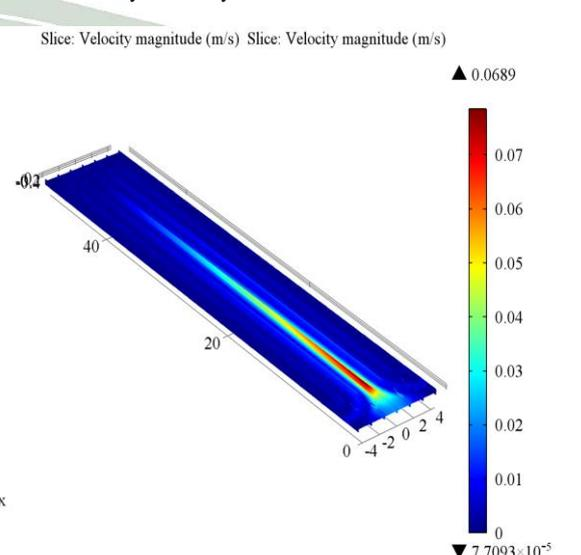
Fig.19. Gas diffusion layer velocity distribution at 0.65 V
