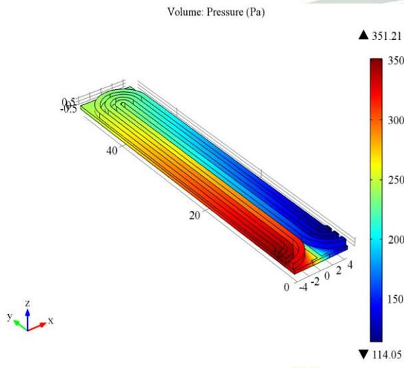
Fig.10. Gas diffusion layer pressure distribution at 0.35 V
