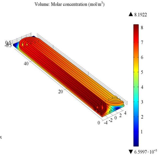
Fig.24. Cathode oxygen concentration at 0.55 V
