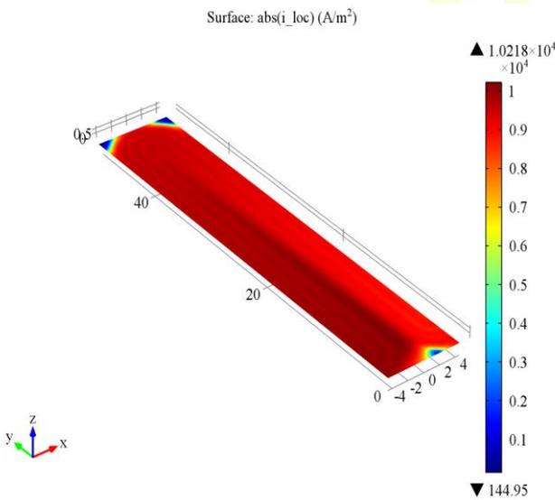
Fig.5. Membrane current density at 0.45 V
