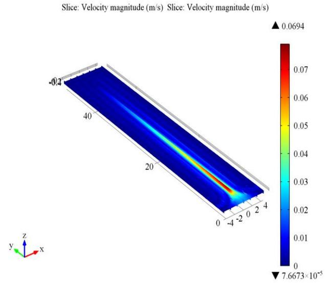
Fig.18. Gas diffusion layer velocity distribution at 0.55 V
