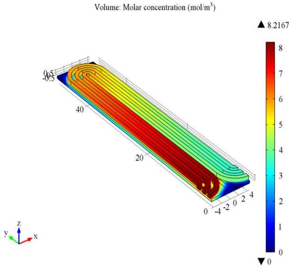
Fig.21. Cathode oxygen concentration at 0.25 V
