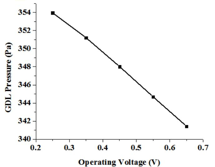
Fig.14. GDL pressure at different voltage level
