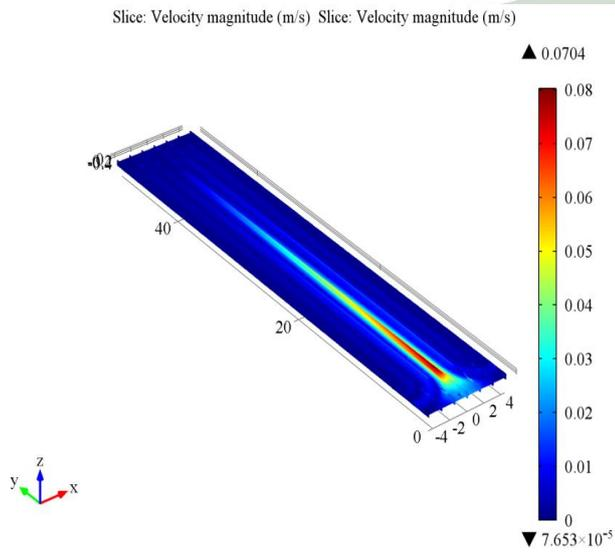
Fig.16. Gas diffusion layer velocity distribution at 0.35 V
