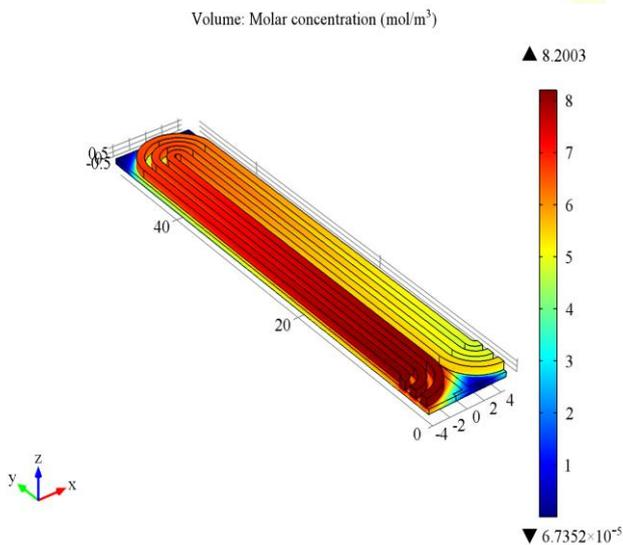
Fig.23. Cathode oxygen concentration at 0.45 V
