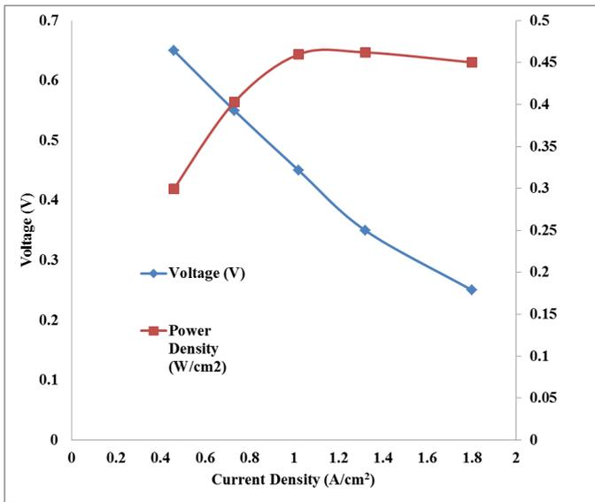
Fig.27. Polarization curve
