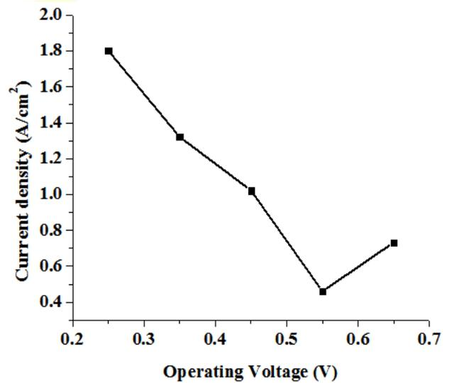
Fig.8. Membrane current density at different voltage level
