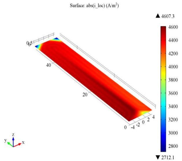
Fig.6. Membrane current density at 0.55 V
