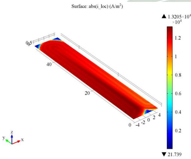
Fig.4. Membrane current density at 0.35 V
