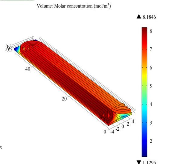
Fig.25. Cathode oxygen concentration at 0.65 V
