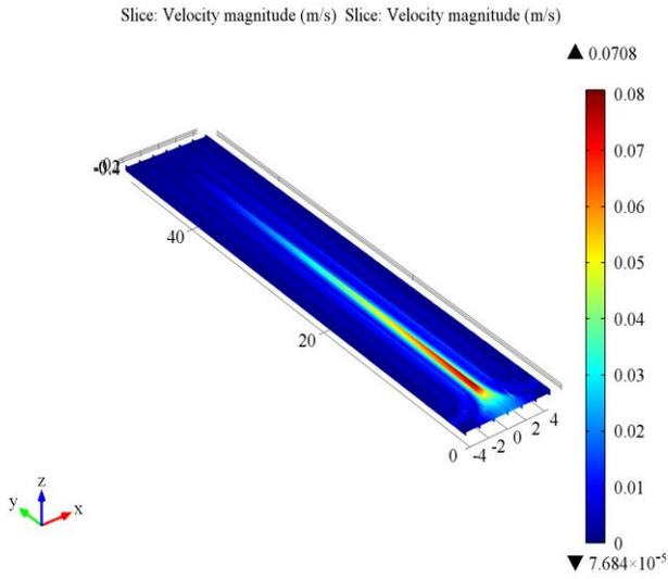
Fig.15. Gas diffusion layer velocity distribution at 0.25 V
