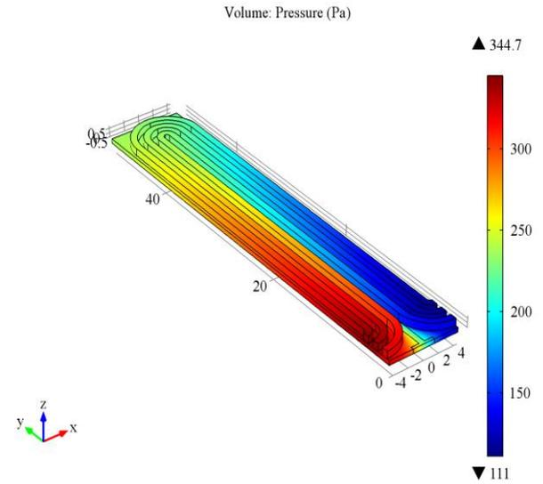
Fig.12. Gas diffusion layer pressure distribution at 0.55 V
