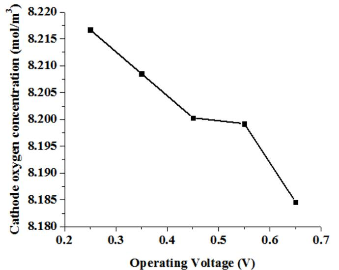
Fig.26. Cathode oxygen concentration at different voltage level
