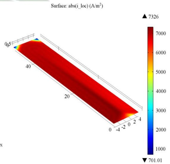
Fig.7. Membrane current density at 0.65 V
