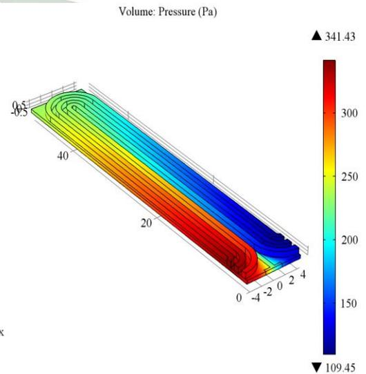
Fig.13. Gas diffusion layer pressure distribution at 0.65 V
