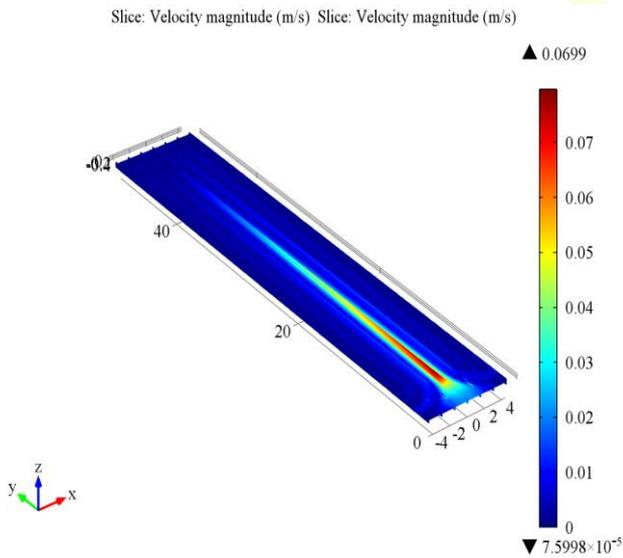
Fig.17. Gas diffusion layer velocity distribution at 0.45 V
