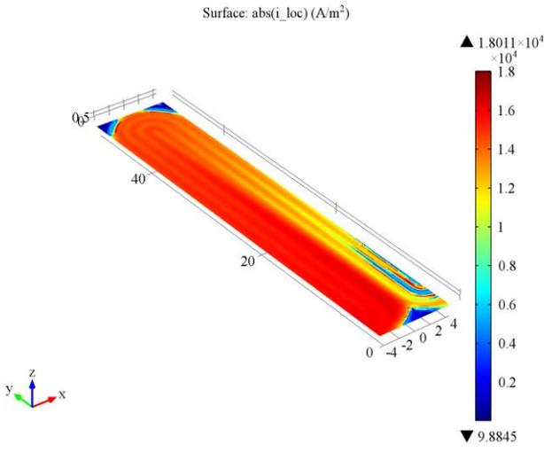
Fig.3. Membrane current density at 0.25 V
