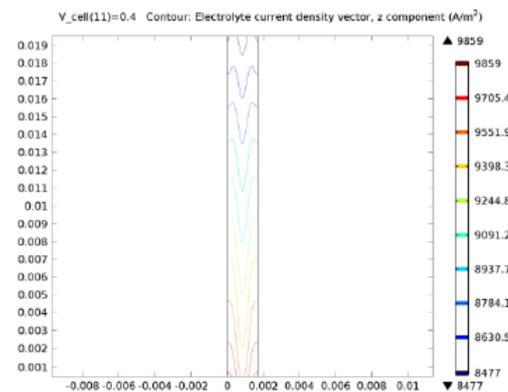
Fig. 4. Ionic current in the polymer membrane at 0.4 V
