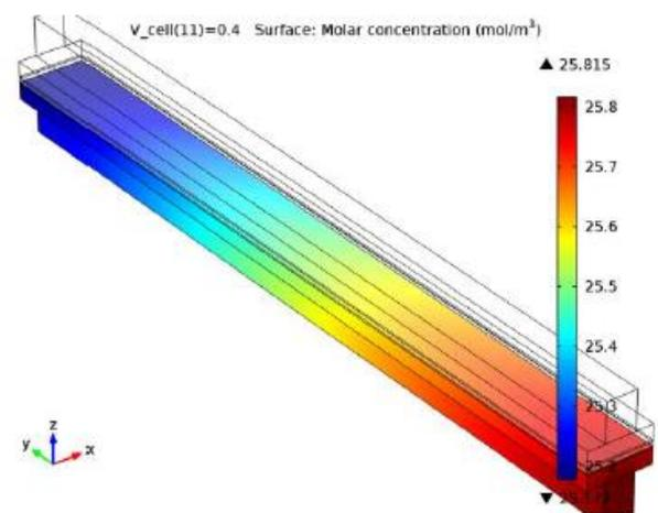
Fig.5. Hydrogen concentration at the anode in the cell at 0.4 V
