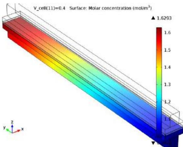
Fig.7. Water concentration on the anode in the cell at 0.4V
