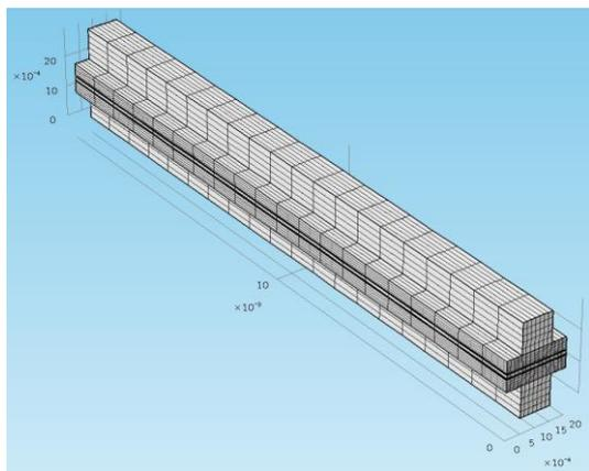
Fig.2. Mesh model of single flow channel PEM Fuel Cell
