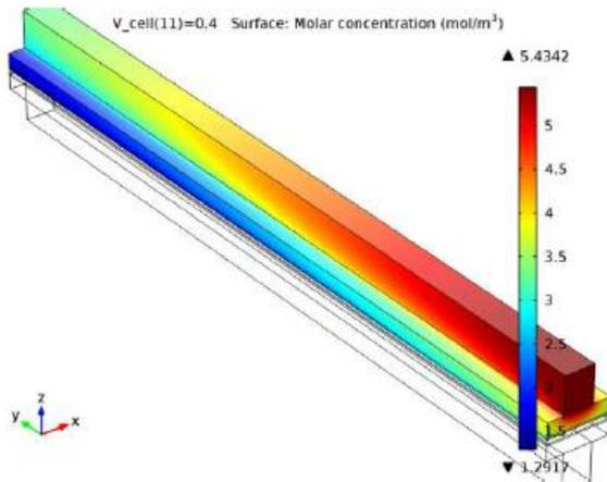
Fig.6. Oxygen concentration at the cathode in the cell at 0.4V
