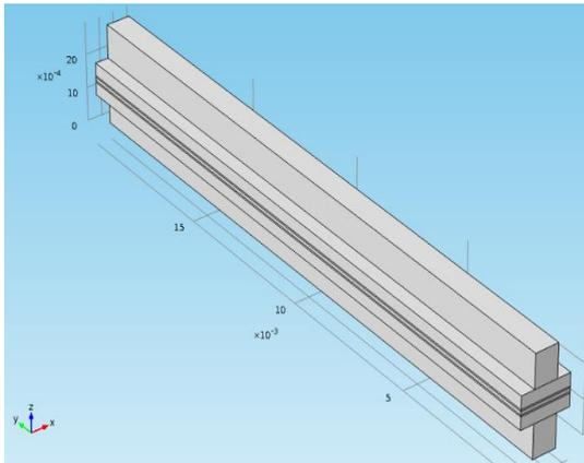
Fig.1 Isometric model of single flow channel PEM Fuel Cell
