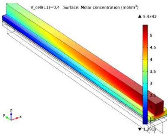
Fig.8. Water concentration at the cathode in the cell at 0.4 V
