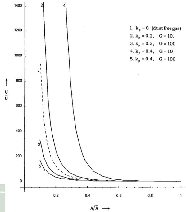
Fig. 1. Variation of shock velocity with channel cross-section for different values of  $k_p$  and  $G$
