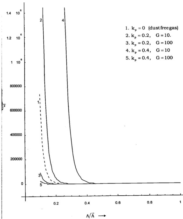
Fig. 3. Variation of pressure just behind the shock with channel cross-section for different values of  $k_p$  and  $G$
