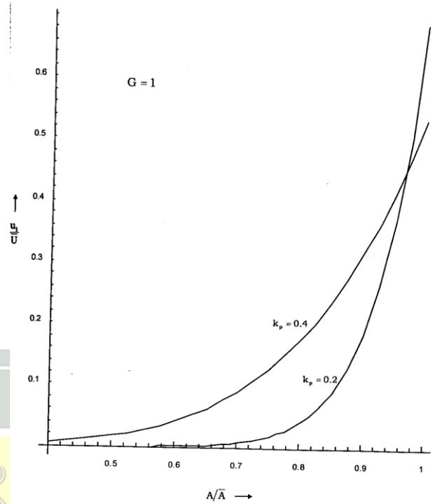
Fig. 5. Variation of fluid velocity just behind the shock with channel cross-section for  $G = 1$
