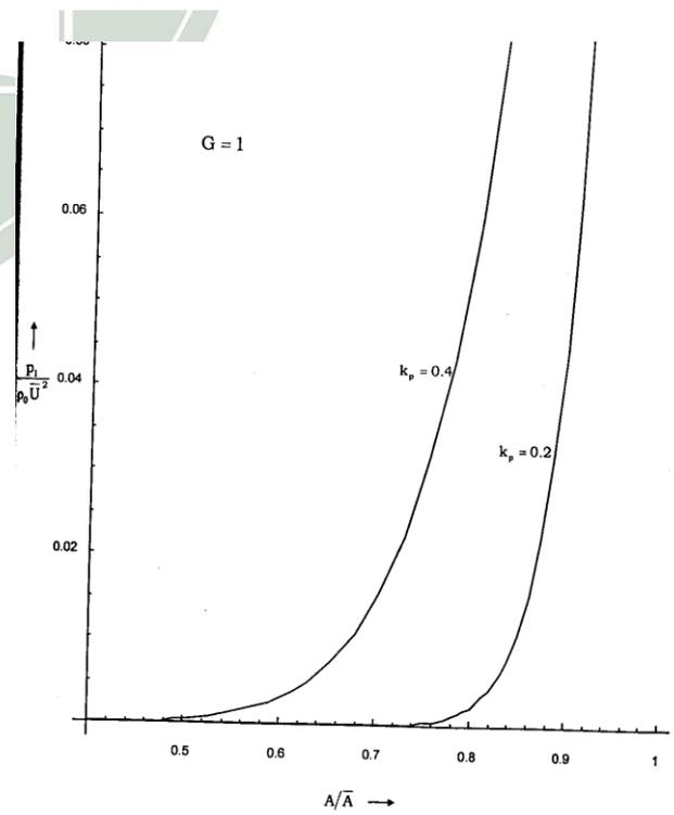
Fig. 6. Variation of pressure just behind the shock with channel cross-section for  $G = 1$
