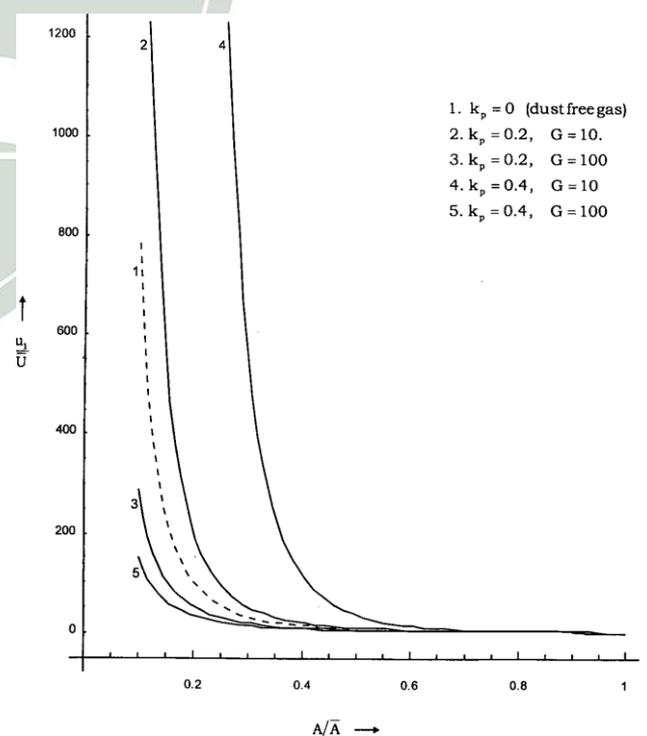
Fig. 2. Variation of fluid velocity just behind the shock with channel cross-section for different values of  $k_p$  and  $G$
