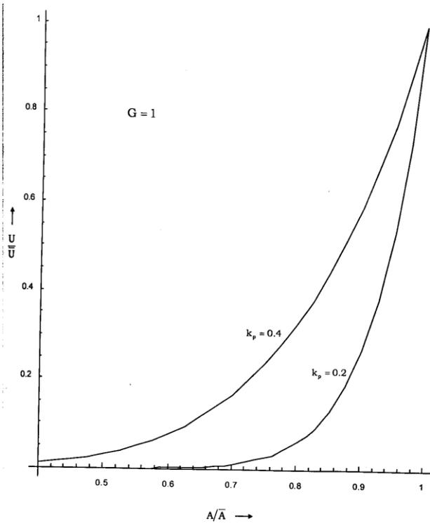
Fig. 4. Variation of shock velocity with channel cross-section for  $G = 1$
