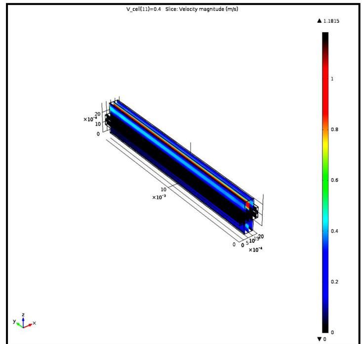
Fig.6. Reactant gases velocity distribution in GDL at 493K
