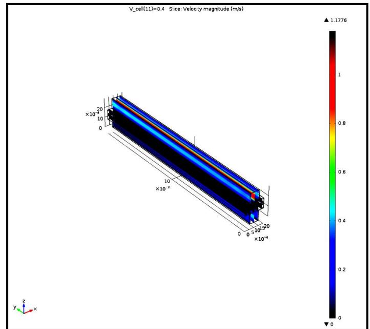
Fig.5. Reactant gases velocity distribution in GDL at 483K
