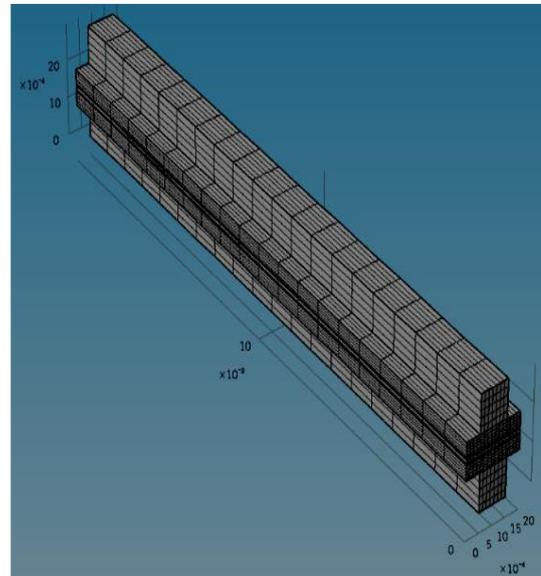
Fig.2. Single flow channel high temperature PEMFC Mesh model
