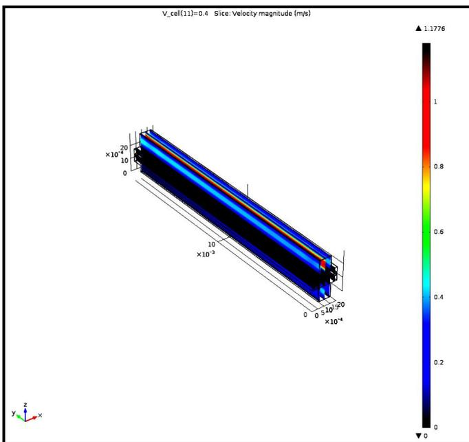
Fig.4. Reactant gases velocity distribution in GDL at 473K
