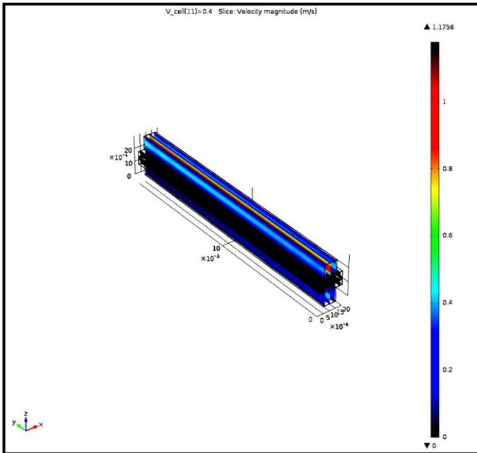
Fig.3. Reactant gases velocity distribution in GDL at 463K
