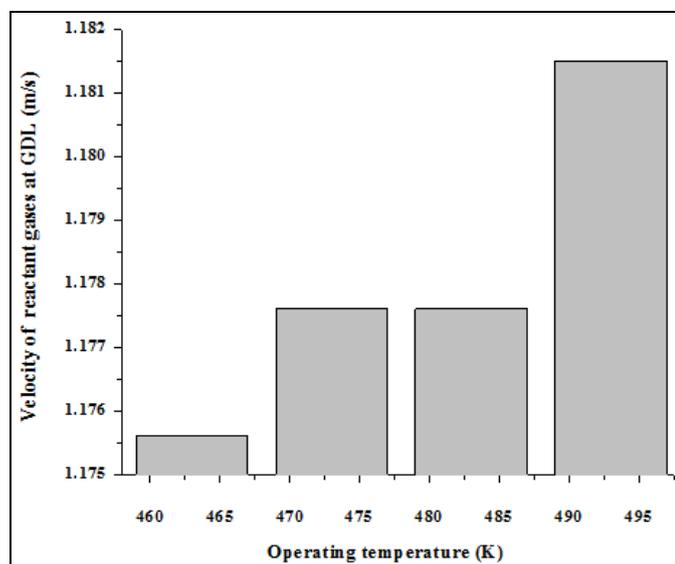
Fig.7. Effect of reactant gases velocity distribution at various operating temperatures
