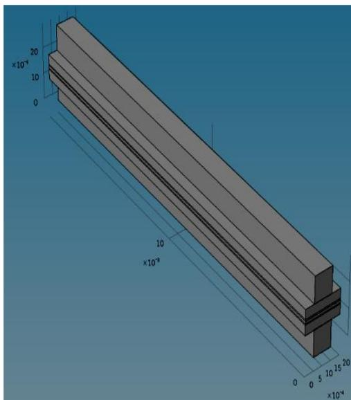
Fig. 1. Isometric model high temperature single flow channel PEMFC
