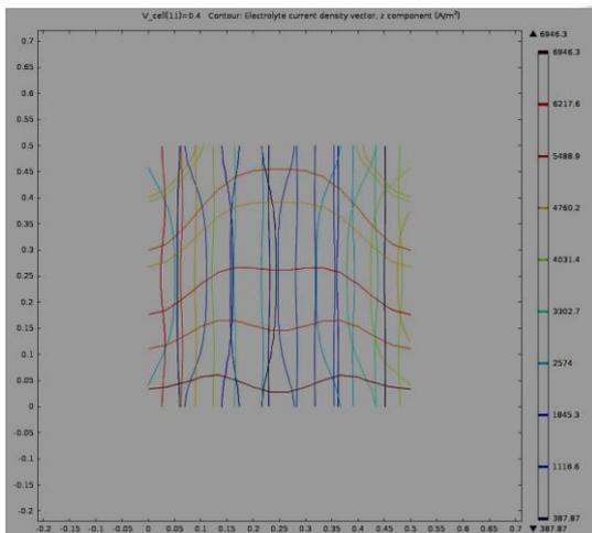
Fig.6. Membrane current density at 220°C
