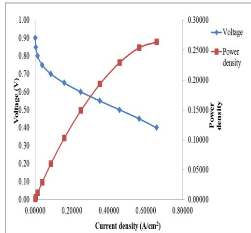
Fig.7. Performance curves at 190°C operating temperature
