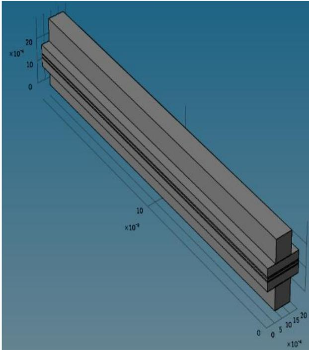
Fig. 1. High temperature single flow channel PEMFC isometric model
