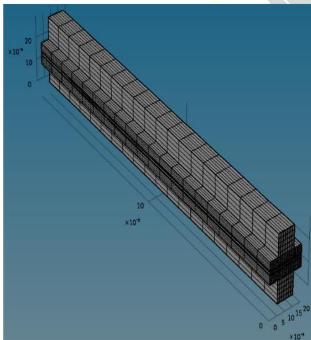
Fig.2. Mesh model of high temperature single flow channel PEMFC
