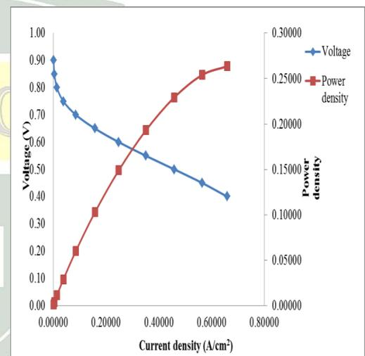
Fig.8. Performance curves at 200°C operating temperature
